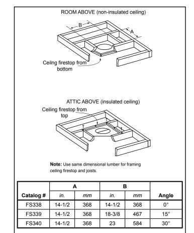
Figure 8.5 Installing the Ceiling Firestop
